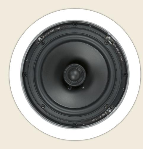
The A-605/70 is the budget-minded answer for both residential and commercial in-ceiling speaker applications. The A-605/70 employs a polygraphite woofer cone and a soft dome tweeter for great sound on a budget. Other amenities include a UL listed integral rear enclosure and a built-in multi-tap transformer, enabling the A-605/70 to be used with either 8 Ohm or 70/100 Volt audio systems. The A-605/70 provides full-range performance while exceeding building code compliance.
