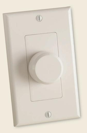
The VLC-100 is an interior decora-style, impedance-matching volume control. Designed to be mounted directly into a standard junction box, the VLC-100 provides a safe operating load to the multi-room audio amplifier and is very easy to operate. A radial-type volume control, the VLC-100 can handle up to 100 Watts per channel and up to 16 pairs of speakers. Five trim colors are included with the VLC-100: Black, Brown, Almond, Bone and White.
