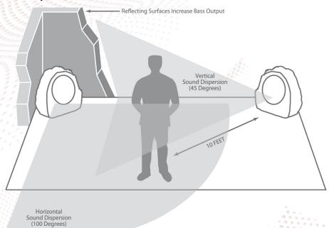
R8 outdoor rock speakers are designed to be placed on the ground with the grille facing the listening area. Speaker drivers are angled upward to provide proper vertical sound dispersion for listeners standing 10 feet or more away. Sound coverage in the horizontal plane is 100-degrees. Too great a distance between any two speakers will create a dead spot. When in doubt use additional speakers to ensure adequate sound coverage.
