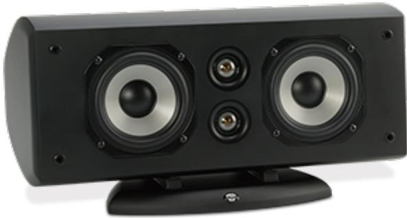
At first glance one might say, "Wait a minute, there's one too many tweeters". But the dual tweeter design of the AC-525 allows a lower crossover point to be used between the tweeters and mid-woofers. The result is better control of the off axis horizontal response and reduced lobbing as compared to a single tweeter center channel design. Not to mention the ingenious swivel stand makes aiming the AC-525 at the listening position a snap.
