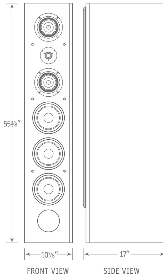
*Cabinets are constructed of ¾-inch high density fiberboard and feature an extensive internal bracing system which virtually eliminates cabinet resonances. This method of construction reduces sound coloration. The thickness of the front baffle also prevents excess acoustic radiation.*
