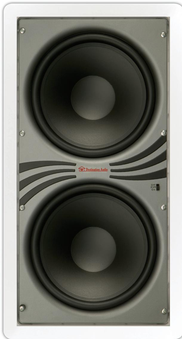
*The SW8 features two eight-inch poly graphite woofers. Poly graphite is used due its stiffness, low mass and self damping properties, the combination of which allows a virtually uncolored presentation of acoustic material. A powerful magnet and extended voice coil give the woofers high excursion capability, which ensures dynamic and accurate audio reproduction.*
