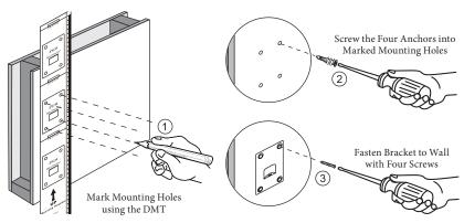
Once all drywall anchors are in place, place the mounting bracket in position, paying careful attention to the bite direction of the bracket (see illustration on page 5). The bite direction of both brackets faces outward from the center of the speaker. Use a screwdriver or drill-driver and four screws per mount to fasten each bracket to the wall securely.
