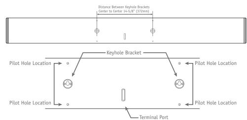
The Ultra-3 soundbar speaker is designed to be used as a LCR (Left-Center-Right) speaker with flat-panel TVs such as plasma and LCD monitors. This will usually dictate placing the speakers below or above the TV. The Ultra-3 speaker sounds best when placed with the s ut optional mounting to TV using universal brackets to accommodate articulating TV mounting brackets is also possible.
